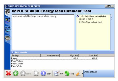
Figure 3-1. Ansur Test Guide Window
