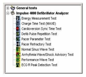
Figure 2-4. Impulse 4000 Test Explorer Window
