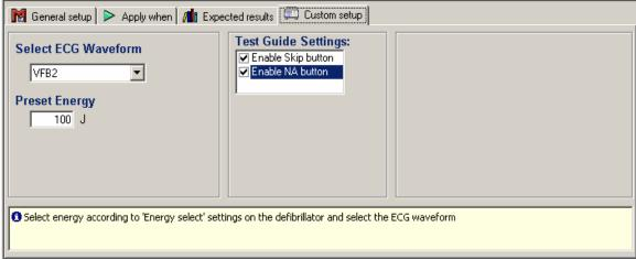
Figure 4-6. Custom Setup Page for Energy Measurement Test Elements
