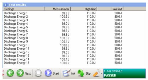
Figure 3-2. Defibrillator Charge and Discharge Test Results
